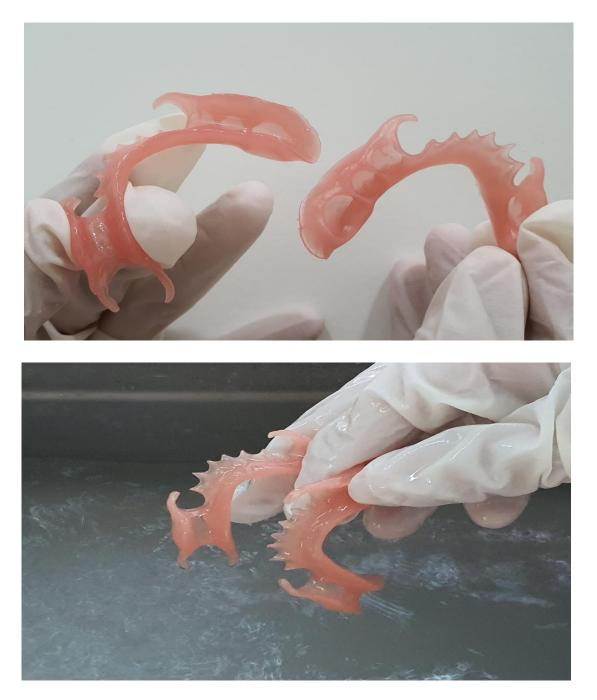
: If there is residual resin, clean for additional 10 seconds using IPA and ultrasonic cleaner.
