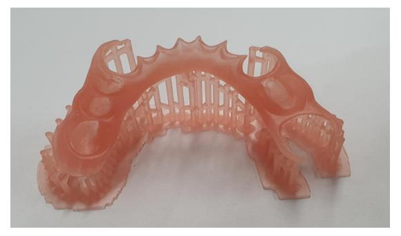
: If the support is generated by the SW which can not control the contact point size between support and flexible denture, cut the support using a nipper.
