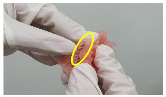
: When removing the support by hand, remove the support around the clasp part first, which is easily damaged.
