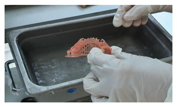
: Wash off the residual resin on the surface of the Flexible Denture Base using IPA(alcohol 99%) and ultrasonic cleaner. : Washing time should be around 30 seconds.
