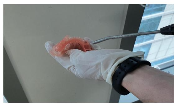
: Blow out the IPA on the surface using an air gun.
