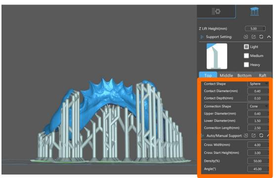
: If you are available to use the SW that can control the detail values of support, reduce the contact diameter to about 0.4mm.
