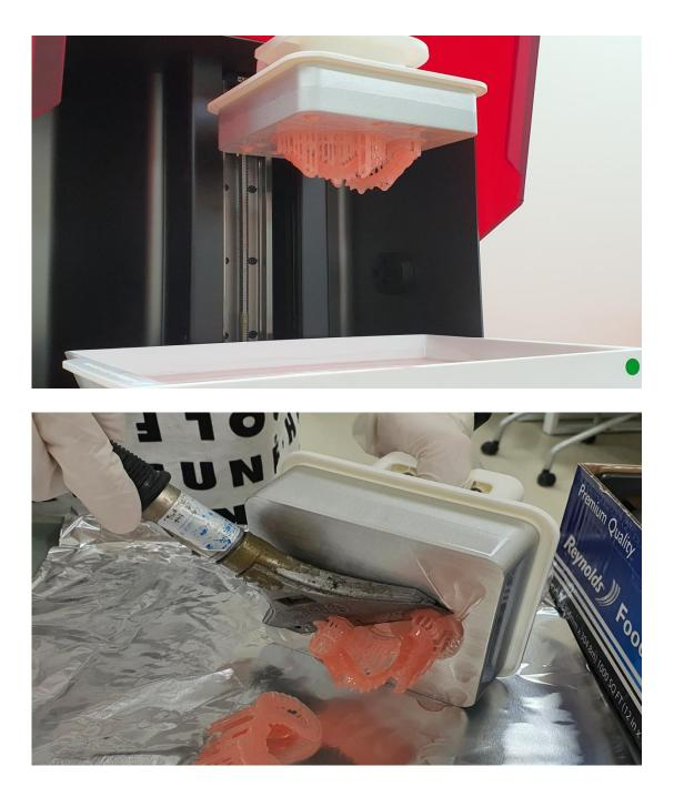
: Detach the printed Flexible Denture Base from the build plate of the 3D Printer with tool like the picture above.
