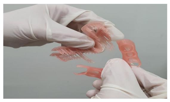
: Gently tear off the support around the rest of border area.
