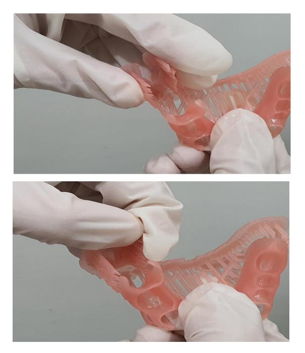
: If the contact Diameter is set to 0.4mm, you can remove support from flexible denture easily by hand.
