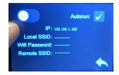
Now toggle the network type. (While WiFi is shown as an option, there is no WiFi hardware inside the printer, so you must use an ethernet cable.) Push the switch in the upper left of the touch-screen to enable the ethernet connection. If you see an IP address
