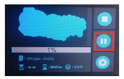
For the first print/new model, it is a good idea to pause the printing after around 30 minutes to confirm that the first layers stuck to the build platform.
