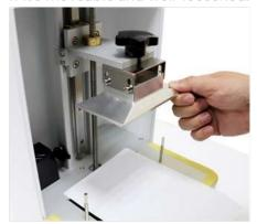
**Step 4→** Click 【Z-AXIS】 button to start the calibration process.
