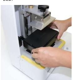
Step 2→ Put 1 piece of A4 paper on the LCD platform.
