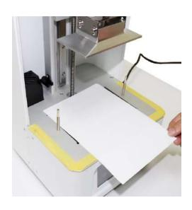
Step 3→ Loosen 4 screws on both sides of the build platform.
