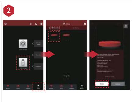
Open the "Print" tab, and choose "USB Storage" to open the file storage path. Select your dual extrusion file to check the printing parameters and settings. Press "Print" to start printing the test file.
