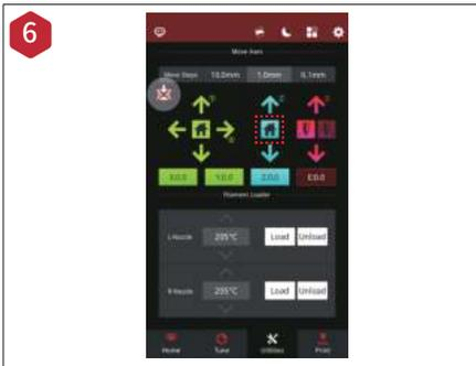
Tap the "Utilities" tab, and press the Z Homing button. Press OK for the print bed to begin to "Home" to the origin position. This will allow you to access your accessory packages.
