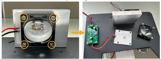
**Step 7:** Remove the red and black wires marked on the LED driver board.
