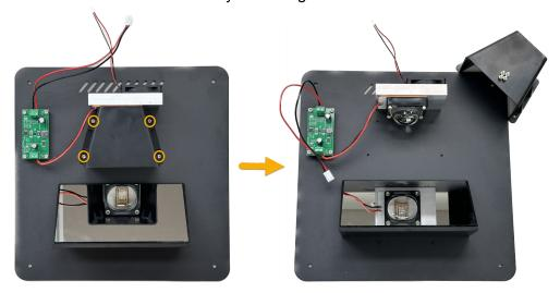
**Step 6:** Remove the LED lens frame by loosening the 4 screws.
