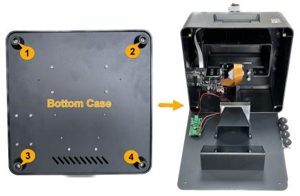
**Step 4:** Unplug the LED connector and Fan connector and remove the bottom case.
