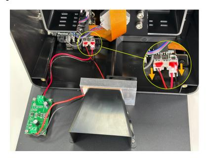
**Step 5:** Remove the black lens hood by loosening the 4 screws.
