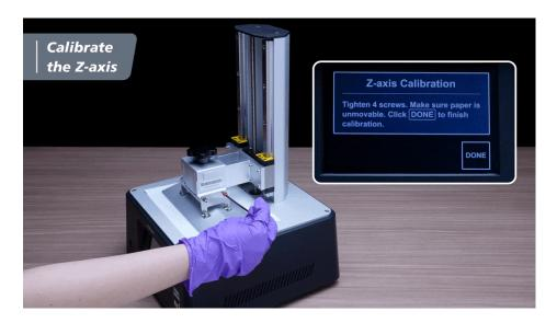
**Step 8:** Double-Check Z-axis Calibration
