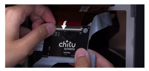
**Step 7:** Turn the 3D printer upright. Remove the black electric tape placed around the LCD. Then, remove the LCD. Use a blade for assistance, if necessary.
