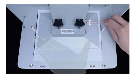
Step 8: Double-Check Z-axis Calibration
