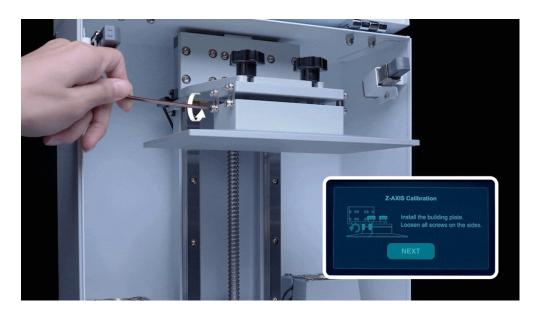
Step 3: Loosen the Screws
