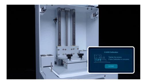
Once the plate has retracted, remove the A4 paper.
