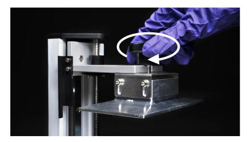
**Step 4:** Use a wrench to loosen all 4 screws present on the sides of the building plate. After loosening it, make sure to double-check to see if the plate is loose and movable.
