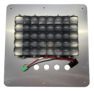
**Step 2:** Connect the LED cable to the mainboard.
