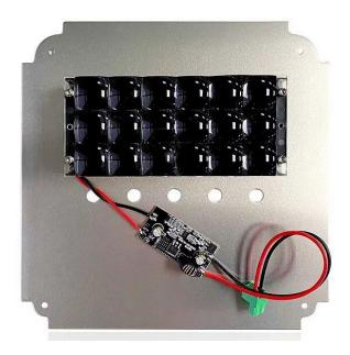
**Step 2:** Connect the LED cable to the mainboard.
