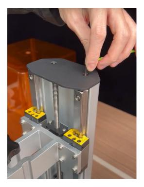
Step 7: Unscrew the T-plate by loosening the 8 screws.
