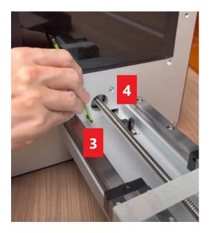
Step 12: Remove the Z-rod from the printer.
