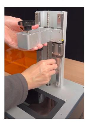
Step 8: Spin the Z-rod clockwise to lift and remove the T-plate.
